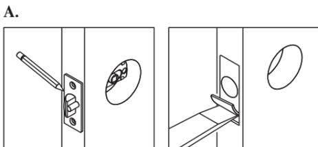
a. Insert latch in hole, mark outline of faceplate and chisel 5/32" (4mm) deep.
