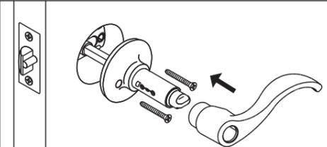
Install installation screws ; then, pushing handle in until catch clicks.
