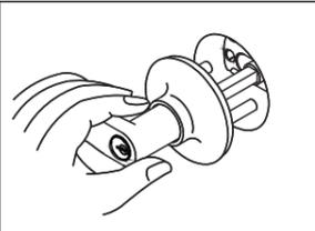
Insert spindle through latch. Press flush against door.
