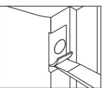
b. Measure one half of door thickness from door stop and mark vertical centre line of strike. Drill 1" (25mm) hole 1/2" (13mm) deep at intersection of horizontal and vertical line of strike. Match screw holes on strike with centre lines on jamb. Mark outline and chisel 1/16" (1.6mm) deep for strike.
