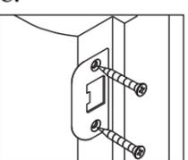
c. Install strike and tighten screws.
