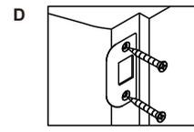
Adjustable tang on strike permits bending in or out to eliminate too loose fit between door and door stop.
