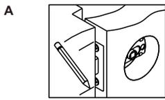
Close door until latchbolt touches jamb to locate strike in jamb and center line of strike. Open door and extend line from mark to door stop. Measure one half of door thickness from door stop and vertically mark drill point center for strike.
