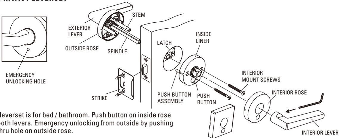
Privacy lever set is for bed / bathroom. Push button on inside rose to lock both levers. Emergency unlocking from outside by pushing button thru hole on outside rose.
