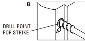
Drill 1" (25.4mm) hole 1/2" (13mm) deep in door jamb on drill point for strike.
