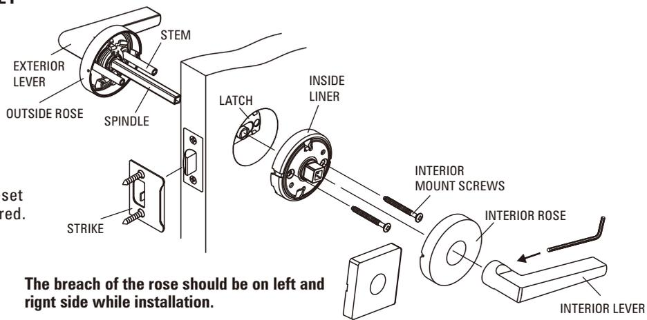
Passage lever set is for hall / closet doors where no locking is required. Depress lever to latch door.
