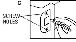
Match screw holes on strike with center line on jamb. Outline outside edge of strike. Chisel 1/16" (1.6mm) deep for strike.
